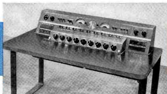
1946. The 25B console is an improved, enlarged version of the 25A, introduced in 1942. For either FM or AM use, the 25B provides two channels and controls two FM or AM programs simultaneously. This new equipment is compact, rugged and modern in appearance. Ease of control, instant accessibility, plug-in cable connections and a frequency response of \pm 1 db, 50 to 15,000 cycles are some outstanding features.
